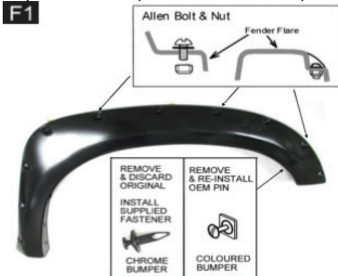
Use torx bit to tighten allen bolt & put firmly on every pocket of the fender flare, shown as top. Remove fastener or pin from rear of bumper. Once the flare lines up, attach and fasten it, shown as bottom.
