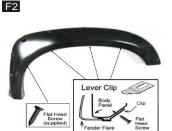
Apply 3 Lever Clips into the mounting slot in flare and secure it to the vehicle with flat head screw, shown as right. Fasten 1 flat head screw into the location, shown as left.
