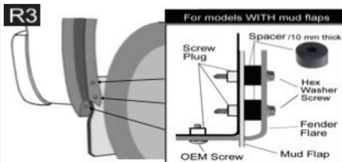
Insert the supplied spacer (10mm) in between vehicle body & flare, apply 2 hex washer screws on top two holes and 1 OEM screw on bottom hole, and secure the flare to the body.
