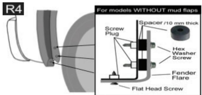
Insert the supplied spacer (10mm) in between vehicle body & flare, apply 2 hex washer screws on top two holes and 1 flat head screw on bottom hole, and secure the flare to the body.
