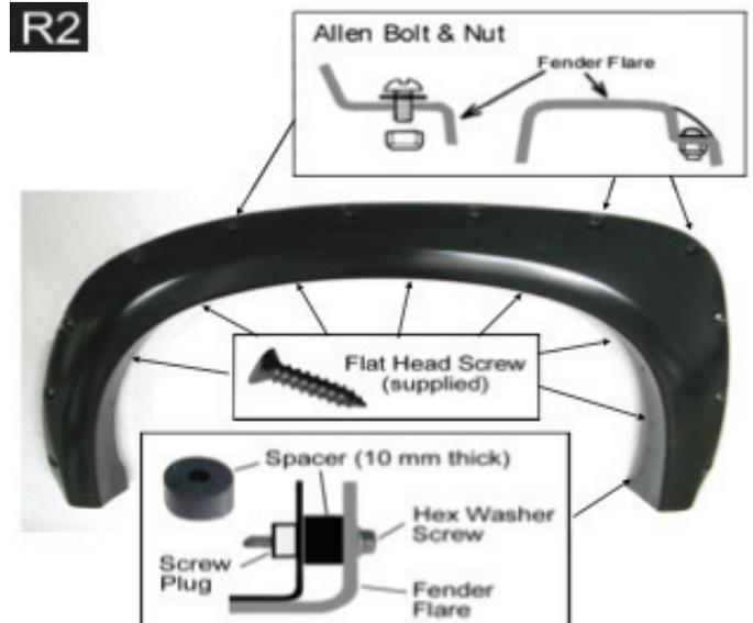
Use tory bit to tighten allen bolt & put firmly on every pocket of the fender flare, shown as top. Fasten 7 flat head screws into the location, shown as center. Insert the supplied spacer (10mm) in between vehicle body & flare, apply 1 hex washer screw to secure the flare to the body.
