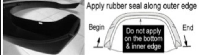
Apply rubber seal to the flare. Start at one end of the flare along the edge that comes in contact with the body panel. Apply pressure on the tape to ensure adhesion, and trim excess rubber seal at the end. To avoid bulge, you may cut a notch in the edge of the rubber seal at the inward angle curve, cut a V out of the outward angle curve.
