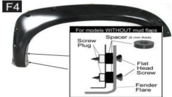
Insert the supplied spacer (5mm thick) in between vehicle body & flare, apply 2 flat head screws to secure the flare to the body as shown.
