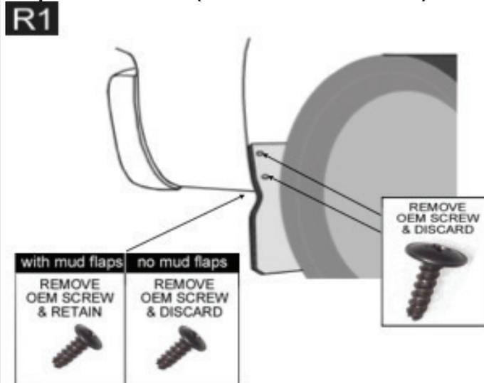
For the models with mud flaps, remove the 2 screws from the mud flap and discard, shown as right. Also remove the screws from the under side of the body and retain, shown as left.
