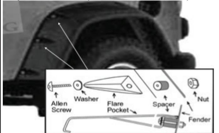
Use right tool to remove rear wheel well skirting and factory fender flares. Place all allen screws, washers through pocket hole, place the spacer on the screw from back side of the pocket as shown. Place the flare on the vehicle with best position and flush against the vehicle. Insert the allen screws through the factory holes on the fender, use hex key to tighten allen screw & put firmly on every pocket of the fender flare. Do not tighten it until all crews have been installed.
