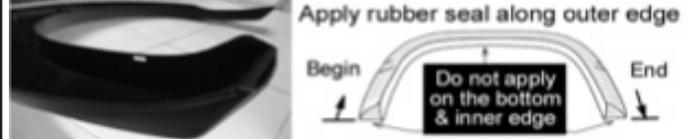
Apply rubber seal to the flare. Start at one end of the flare along the edge that comes in contact with the body panel. Apply pressure on the tape to ensure adhesion, and trim excess rubber seal at the end. To avoid bulge you may cut a notch in the edge of rubber seal at the inward angle curve, cut a V out for the outward angle curve.
