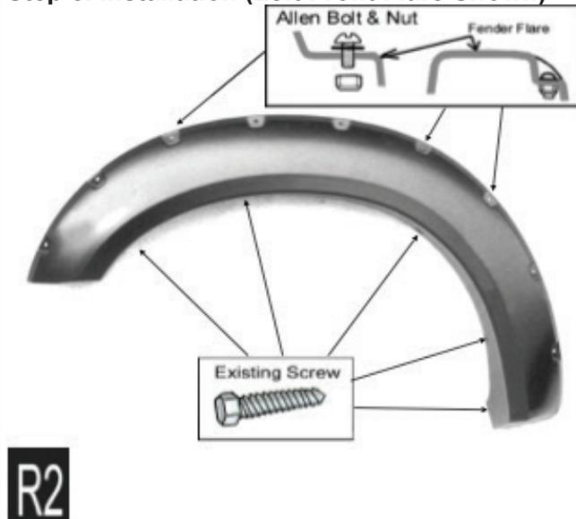
Use torx bit to tighten allen bolt & put firmly on every pocket of the fender flares. **DO NOT OVER TIGHTEN!** Remove 5 existing screws from the vehicle. Place the flare on the vehicle. Re-Install the existing factory screws into the original location that were previously removed. Do not tighten the screws fully until the flare are aligned and extrusive against the body.
