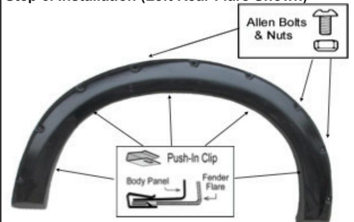
Use torx bit to tighten allen bolt & put firmly on every pocket of the fender flares. Place the flare on the vehicle. Apply 5 Push-In Clips into the mounting slot in flare and secure it to the vehicle as shown.
