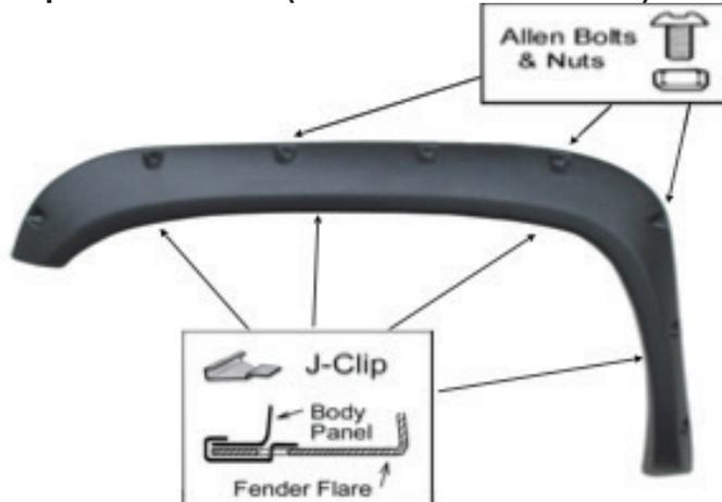
Use torx bit to tighten allen bolt & put firmly on every pocket of the fender flares first. Place the flare on the vehicle. Apply 4 J-Clips into the mounting slots in the flare and secure it to the vehicle as shown.
