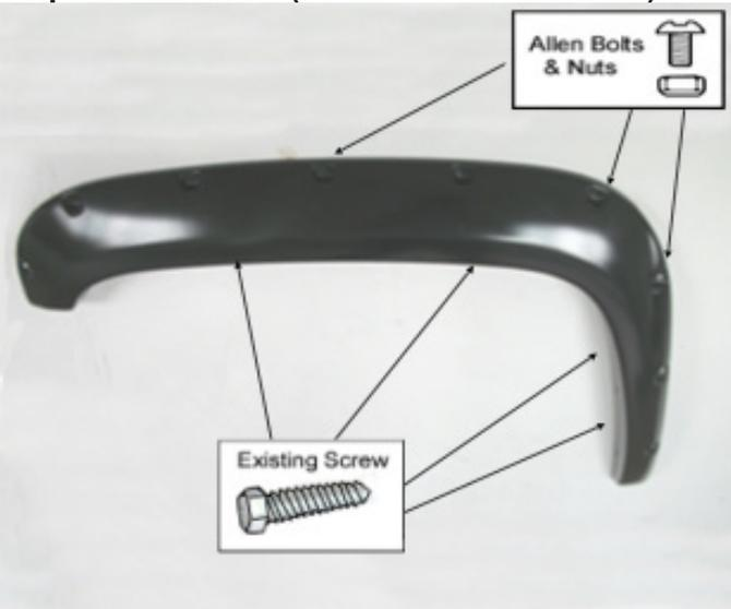
Place the flare on the vehicle. Fasten the existing factory screws into the original location that were previously removed as shown.
