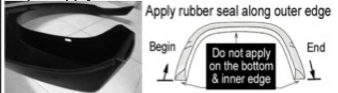
Apply rubber seal to the flare. Start at one end of the flare along the edge that comes in contact with the body panel. Apply pressure on the tape to ensure adhesion, and trim excess rubber seal at the end. To avoid bulge you may cut a notch in the edge of rubber seal at the inward angle curve, cut a V out for the outward angle curve.
