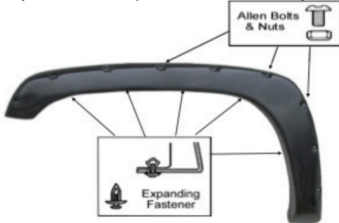
Use torx bit to tighten allen bolt & put firmly on every pocket of the fender flares first. Place the flare on the vehicle. Apply 5 Plastic Expanding Fasteners into the mounting slots in the flare and secure it to the vehicle as shown.
