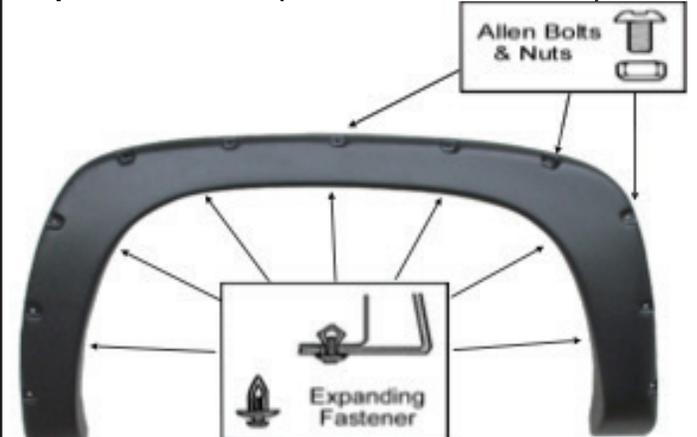
Use torx bit to tighten allen bolt & put firmly on every pocket of the fender flares first. Place the flare on the vehicle. Apply 7 Plastic Expanding Fasteners into the mounting slots in the flare and secure it to the vehicle as shown.
